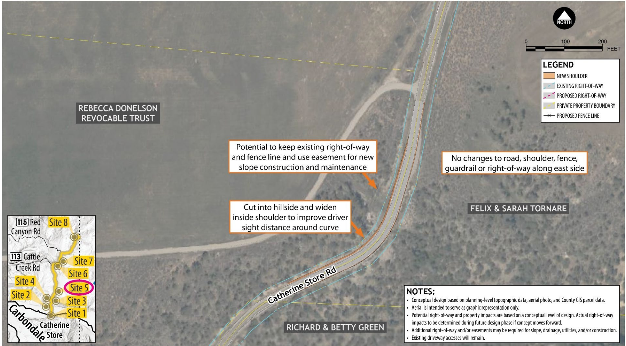
Figure 7. Garfield County Site 5 - Hillside Grading
